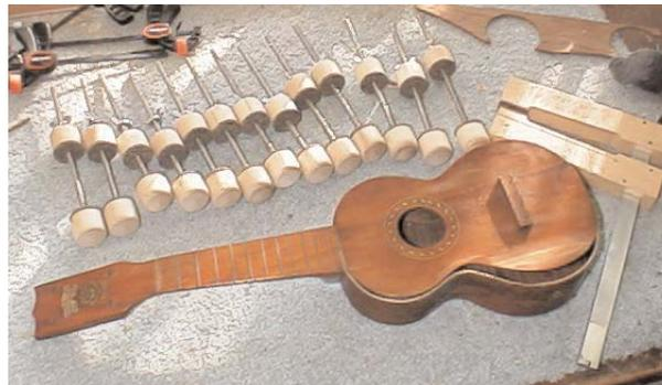
On Day 5 I began gluing koa cleats along the side to keep the splits from opening again. The top left picture shows the cleats later in the day after I took the clamps off. The top right picture shows the glued cracks and small patch.
