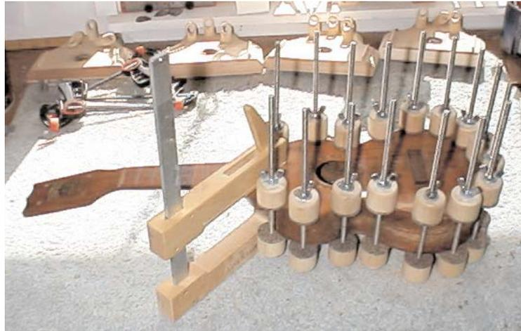
Day 6 was the top gluing day. This is a delicate procedure, because of the thinness of the woods. The sides had to be carefully “pinched in” to fit the top properly, and the clamps couldn’t be tightened too much or it would crush the wood. The whole process took nearly an hour to complete.
