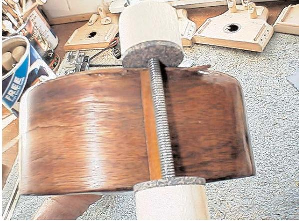
Day 7 showed the results of the top gluing. It all went very well, and I was able to reinstall the 12th fret where the top met the fingerboard.
