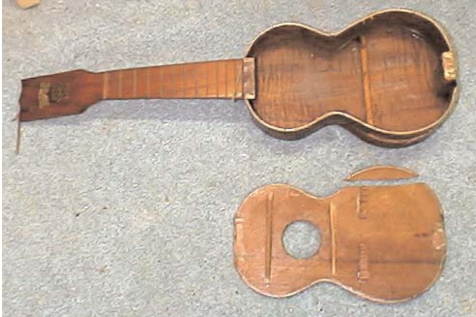
The next day, Day 2, I carefully removed the top and continued my assessment of damages. Because some areas were already open where the glue failed, I was able to take a very small, thin bladed Xacto knife and run it around the edge to pop the remaining glue joints free.
