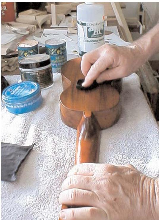
On Day 11, after the tung oil had dried thoroughly, I rubbed out brush marks, bits of dust, and minor scratches using pumice and rottenstone soaked with a special mineral rubbing oil. After nearly 30 minutes of rubbing, I used a beeswax cleaning solution. After rubbing that off, I applied paste wax and polished the ukulele to a fine sheen.
