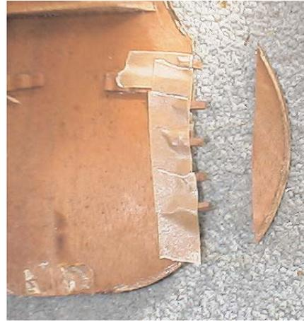
On Day 3, I began the crack repairs. I was able to “pop” the side splits back into place and squeezed glue into the joints. I used special binding tape to hold the cracks together, and mini clamps to keep them in place.
