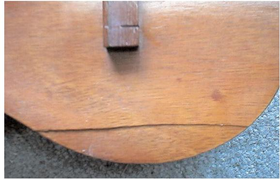
On Day 1, I made a full investigation and assessment of damages. Kumalae ukuleles are known for having almost paper-thin wood on the body, and the split sides and broken top showed this to be true. The large side split had most wood intact, but pushed in, and a little had broken off and was lost.
