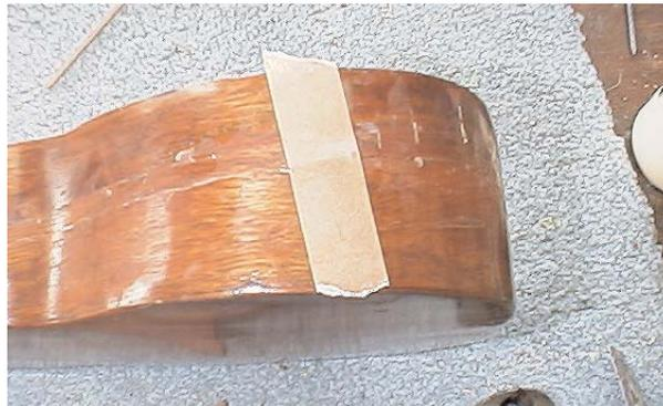
The next day, Day 4, I glued the broken off top piece to the cleats. Again, I used binding tape and mini clamps to hold it in place. Since it was a warm day, the glue dried in a few hours and I was able to remove the tape and clamps. The cleats help strengthen the top and keep the crack from ever opening again.
