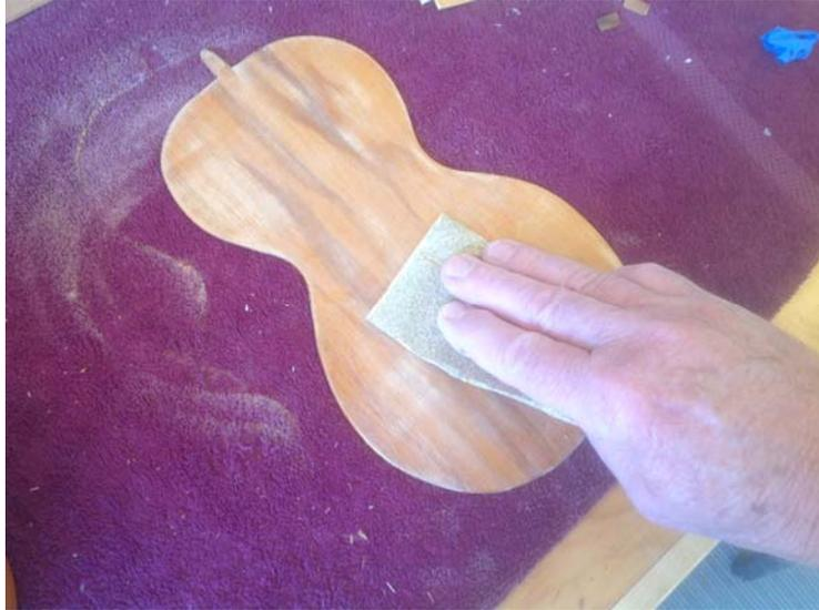
Now with the crack repaired, I needed to sand the back to remove any glue residue. At the same time, I was sanding down the finish so there was no more “frog skin” look.
