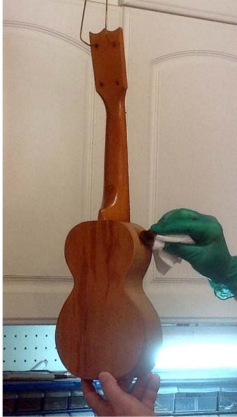
After the stain dried fully, I started the final finishing steps. For four days, I applied four coats of tung oil varnish. I brushed it on, and wiped it off with a lint-free rag so there would be no drips.
