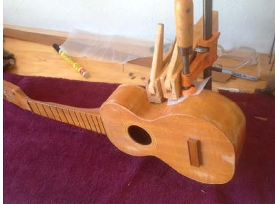
To fix the small crack where the back brace was pushing into the side, I opened it a little and cut into the brace a little with a micro chisel so I could place and glue a small piece of matching koa into the opening.
