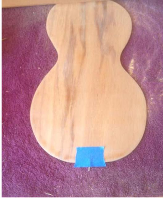
The tail end of the back, where the crack started, had a chip out of it.
