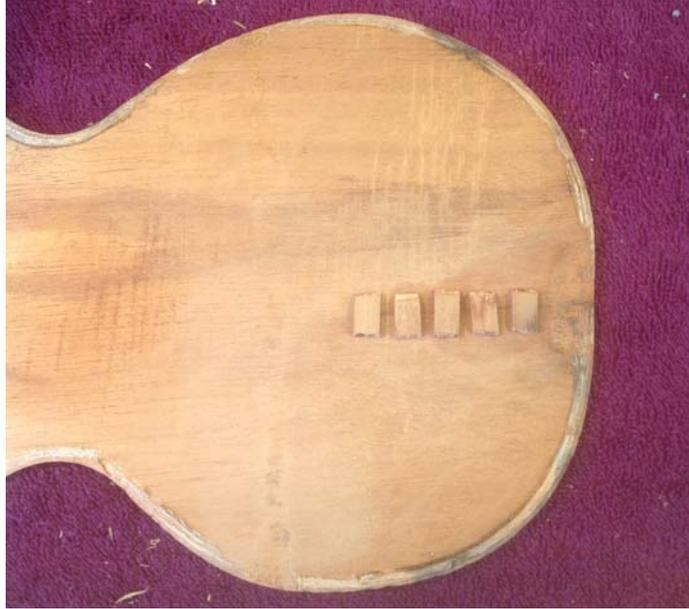
After the glue in the crack dried, I made up some thin cleats of scrap koa and glued them across the length of the crack.
