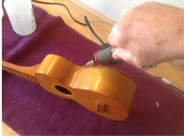
To do a good repair on the back crack and to be able to stabilize it well, I removed the back.
