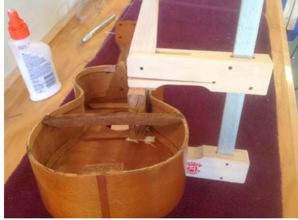
With the back off, I noticed a slight gap in one of the top braces. I slipped an Xacto blade under to see how much of the brace had come loose.
