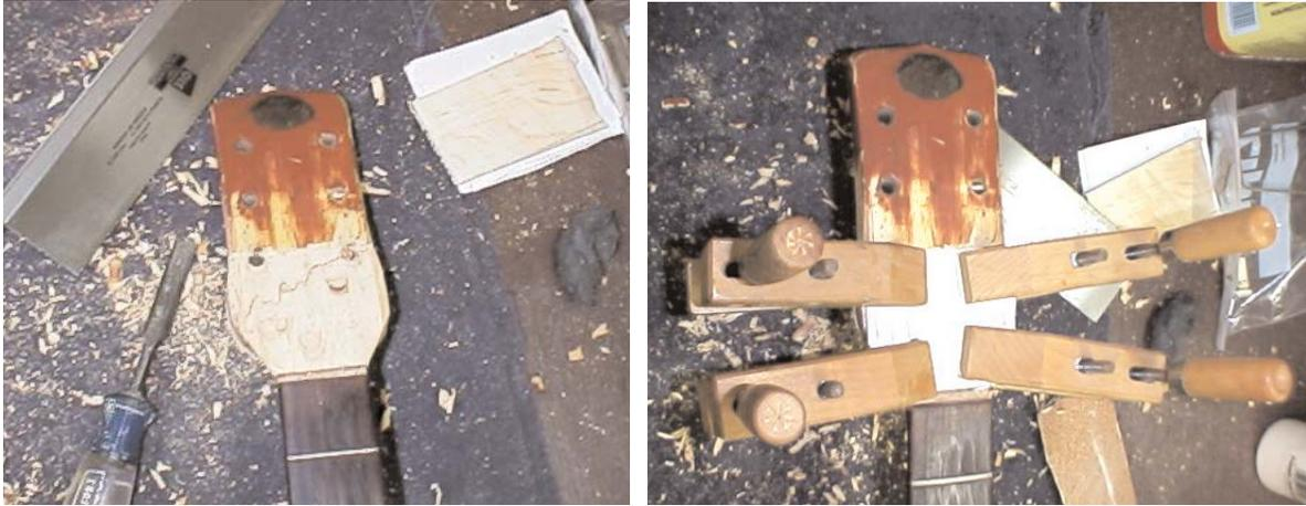
Since the head did not have a lamination on its face, like many guitars have, that helps strengthen it, I wanted to slot the top like I did the back of the head to put a hardwood strengthening piece over the break. This, too, was glued and clamped overnight.
