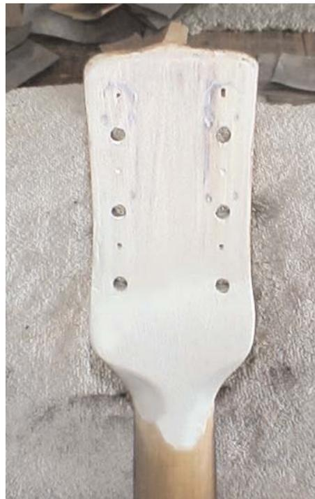
I let the glue set for a few days before starting to put a finish on the head. Because of the new wood, and some of the old wood being exposed, I had to put on a few coats of primer/sealer.
