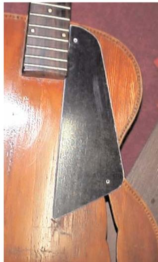
Day 9 saw me working on, and completing, several repair projects. I had put the last coat of color on the head and got it ready for several top coats of tung oil varnish. I also added some coloring to the new purfling tiles and binding, also getting it ready for tung oil.
