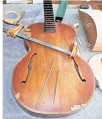
A section of binding was broken off, and several pieces of the unique tiled wood purfling were missing, probably due to the guitar being dropped at one time. There was also a slightly loose section of binding on the upper left bout, which I strengthened with a thin white glue.
