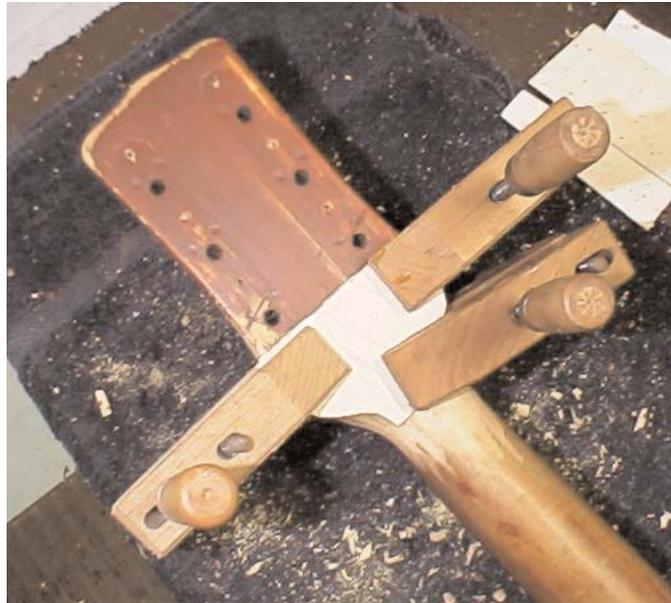
To add more strength, I slotted the back of the head and added a thin piece of maple. Again, I clamped it overnight.
