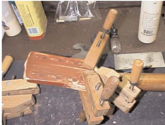
The head was the hardest part of the repair, due to the break having been previously repaired with a kind of all-purpose or airplane glue. With a little heat and judicious prying, it came off fairly easily. In fact it came off so quickly, I was sure that if the guitar had been strung up with heavy gauge strings before it was repaired, the head would have snapped off anyway.
