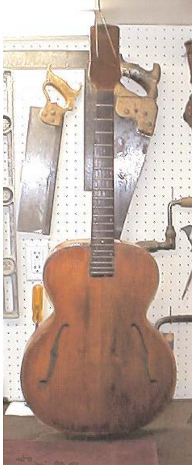
On Day 11, I gave the entire guitar a final sanding, with 320 to 400 grit sandpaper and 0000 steel wool, cleaned it up, then applied a liberal coating of tung oil varnish. After the cleaning of the old wood, the tung oil brought out a nice honey color and a slight gloss to the instrument.
