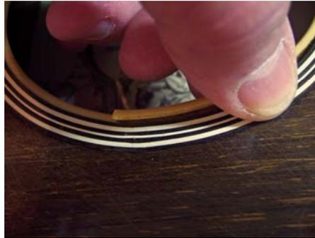
On the first day, I always look over an instrument to see how much work is needed to repair or restore it. This zither was not in bad condition at all. The fingerboard had a few “shrinkage” cracks, a small top crack (almost unnoticeable), and loose sound hole binding. The carrying case covering was peeling off, but easily fixed.
