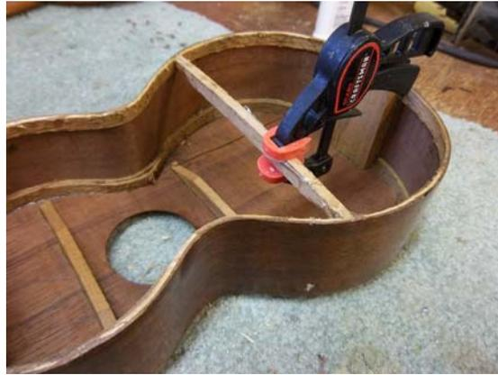
On this day I fixed the back crack. I used special curved violin clamps to pull the sides together to close the crack after applying glue. I also glued and clamped the broken back brace.
