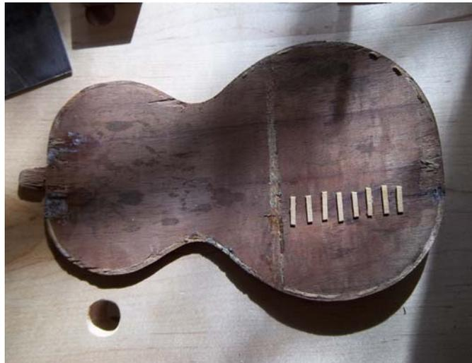
This day I did quite a bit of work on crack repairs. After injecting glue into the cracks, I put pressure on the sides of the top using a cam clamp to close them up. I used the other clamps to keep the top from buckling under pressure.
