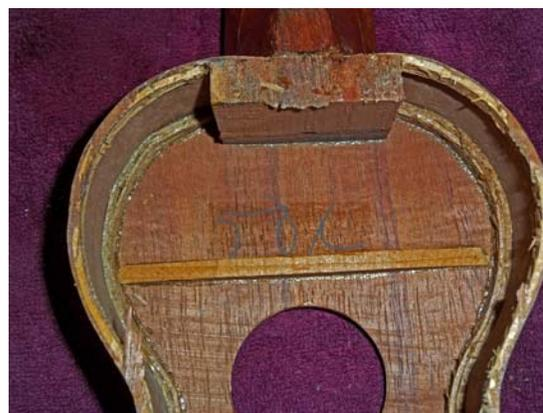
On Day 2, I removed the strings and tuning pegs and began the long process of back removal. Since the back had a couple of small areas where the glue failed, I started steaming around those to soften up the surrounding hide glue, working with both a fine-bladed X-acto blade and a thin artist's palette knife. After a couple of hours, I was able to lift the back from the body.
