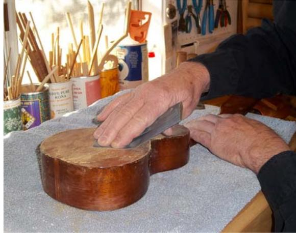
Now that the ukulele is together, I needed to scrape the instrument to take off glue that had squeezed out from the clamping process. Because scraping takes the old finish off, I needed to sand most of the uke to even out the surface so later touch-ups wouldn't look uneven and blotchy.
