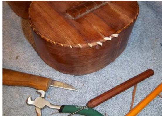
For the next three days, I cut and glued tiny pieces of koa and maple to replace the missing section of rope binding. I could only glue one piece at a time, and wait for it to dry before adding another piece.
