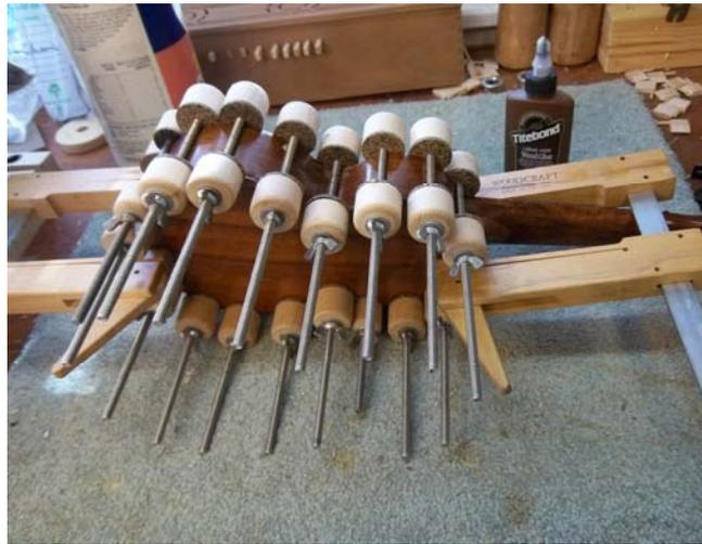
A few days later I began to reassemble the ukulele using a combination of spool and cam clamps.
